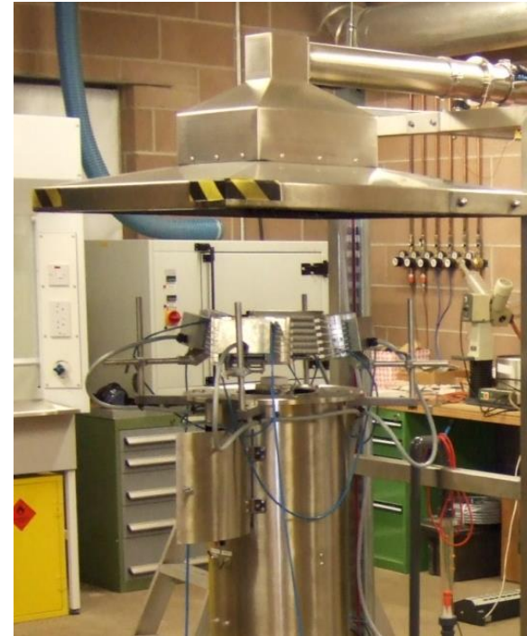
Example of oxygen-controlled tests (FPA)
