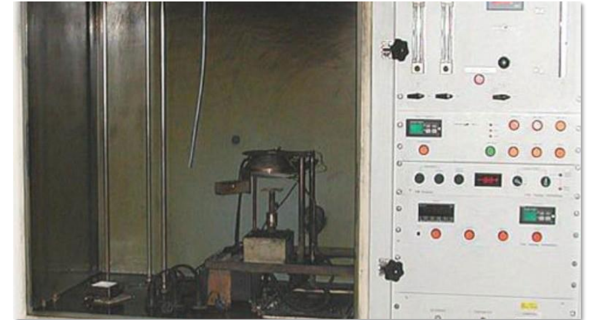
Smoke chamber ISO 5659. Photo © courtesy of Crepim
